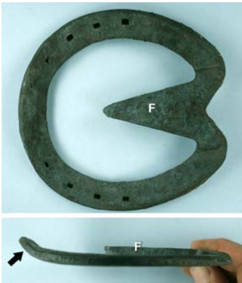
Figure 11-7 The heart-bar shoe. Factory made heart-bar shoes are readily available in a range of sizes and can be shaped to fit most horses. As supplied, the shoe is flat and must be adjusted so that the frog plate (F) is “set up” above the level of the branches of the shoe. The frog plate should be parallel to and 2-3 mm above the level of the adjacent branches of the shoe. The frog support plate of the shoe should apply even pressure over the entire length of the frog. Rolling the toe of the shoe (arrowed), eases breakover of the foot during locomotion, and relieves tension on lamellae weakened by laminitis.
