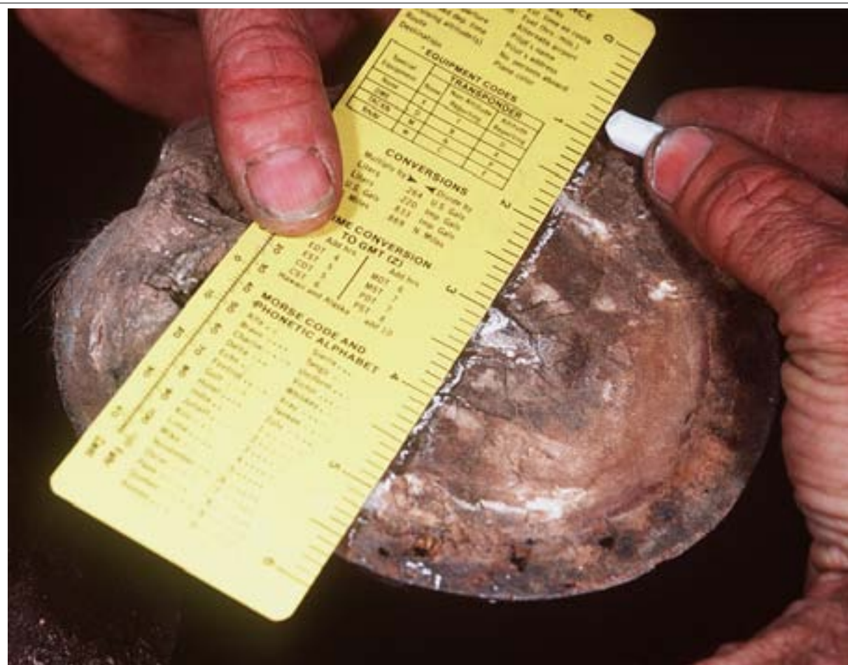
Figure 11-9 Fitting the heart-bar shoe (B).
